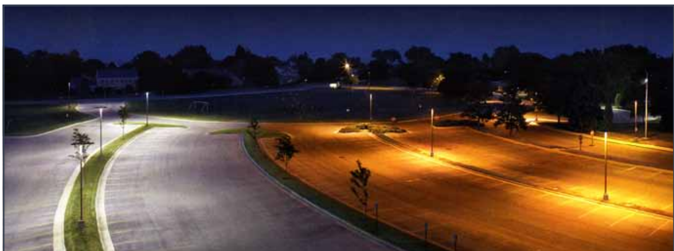
LED lighting (left) uses 90% less energy with a bulb life of 10 times longer than the high pressure sodium lighting (right).
