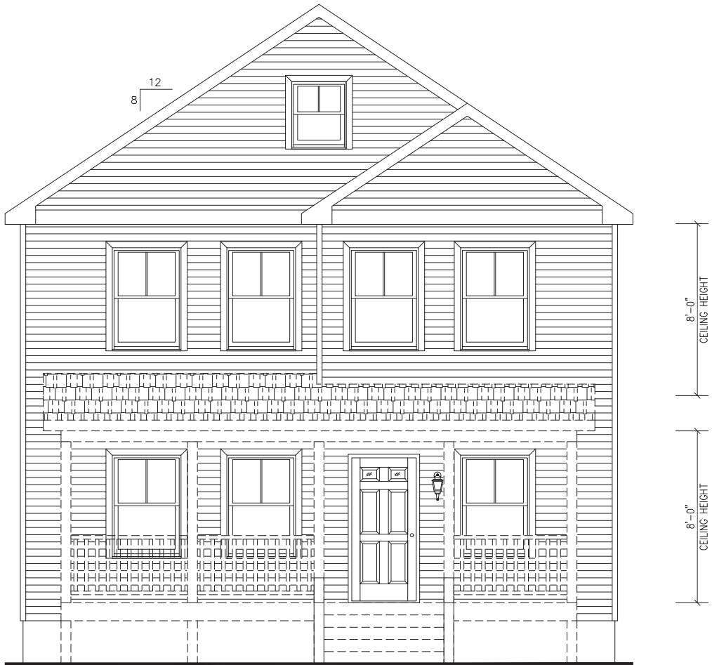
FRONT ELEVATION INDEPENDENT BUILDER'S SITE CONTRACTOR TO PROVIDE ACCESS TO GRADE INDEPENDENT BUILDER'S SITE CONTRACTOR IS RESPONSIBLE FOR DESIGN AND INSTALLATION OF FOUNDATION
