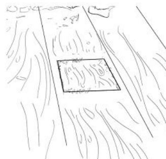
Step 3: Fit a new block of wood in the hole
