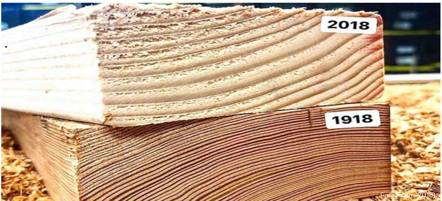
Figure 7.2 - 1918 wood harvested from old-growth forests is dense and durable. It will burn more slowly and is more insect resistant. It is now hard to obtain and if found, expensive. The alternative new-growth wood (the 2018 example) is visibly much less dense and less resistant to moisture and insects. It will require frequent replacement and is less favorable than maintaining historic wood.
