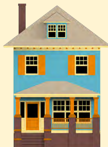
Figure 3.2 - This foursquare house has a boxy shape with triangular and trapezoidal roofs. The overall shape emphasizes verticality as well as the post on piers supporting the porch.
