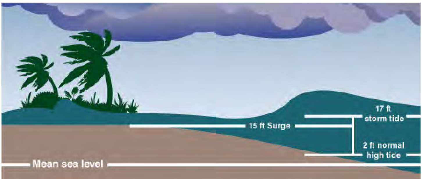
Figure 8.2 - A diagram from the National Oceanic and Atmospheric Association illustrates a storm surge.
