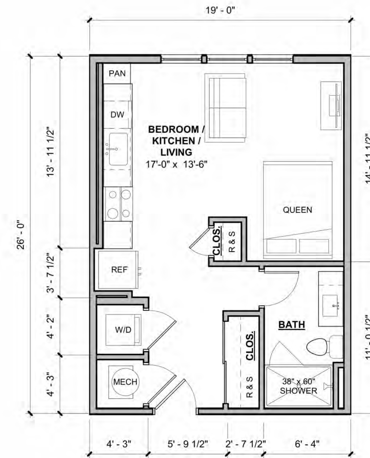
CONCEPTUAL UNIT PLAN - A1 AREA : 520 SF SCALE : 1/4"=1'-0"
