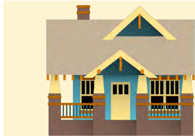
Figure 3.4 - This Craftsman style house has a low pitch roof, but with multiple dormers, decorative brackets, and a chimney that add defining features to the roof.
