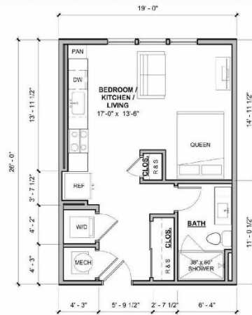
CONCEPTUAL UNIT PLAN - A1 AREA : 520 SF SCALE : 1/4"=1'-0"
