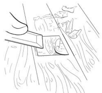
Step 4: Chisel and sand the edges until even
