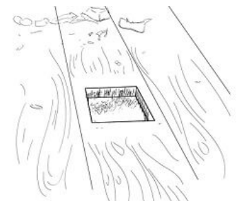
Step 2: Remove the rotten area
