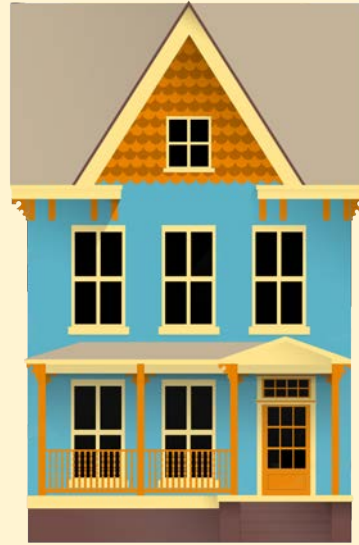
Figure 3.6 - Gingerbread brackets at the roof and porch, turned balusters, and fishscale shingles all add to this building's character.
