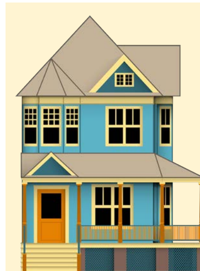
Figure 3.5 - Queen Anne style houses typically have many examples of projections. Here, bay windows, a tower, dormer, and wrap around porch are all considered projections.
